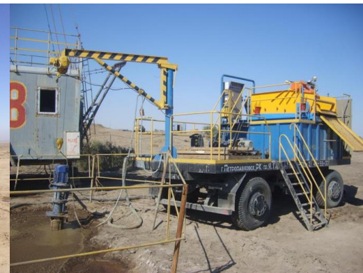
Mobile unit for cleaning drilling mud from drill cuttings
